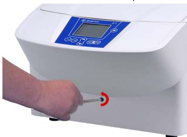
Fig. 12: Manual release of the lid lock
