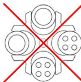
Fig. 6: Permissible and impermissible loading of a swing-out rotor with different tube sizes (example illustration)
