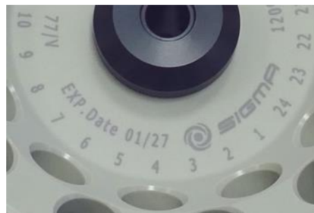
Fig. 4: Different service life – engraving on the bucket/rotor
