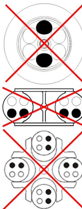
Fig. 7: Permissible and impermissible loading of an angle rotor and a swing-out rotor (example illustrations)
