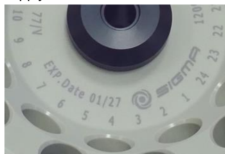
Fig. 5: Different service life – engraving on the bucket/rotor
