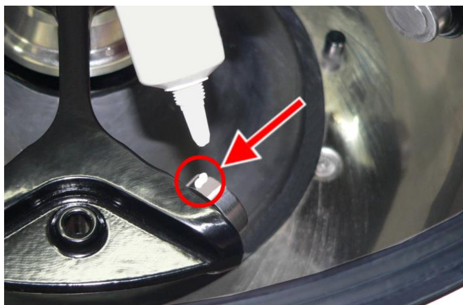
Fig. 13: Sufficient quantity of grease for one bolt
