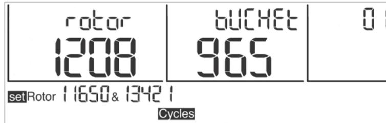
Fig. 28: Cycle display for rotor 11650 and bucket 13421
