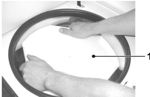
*Fig. 9: Removal of the transport safety device (example)*
