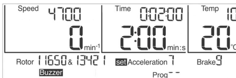
Fig. 24: Preselection of a curve; here: preselection of an acceleration curve
