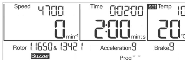
fig. 21: Setting the temperature
