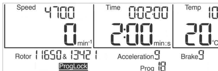
Fig. 27: The program lock "ProgLock" is activated
