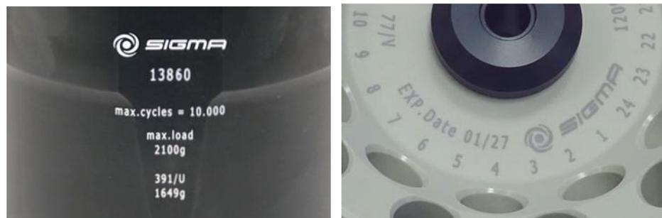
Fig. 5: Different service life – engraving on the bucket/rotor
