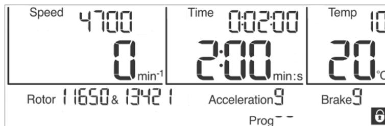
Fig. 30: "Padlock" symbol indicating an activated input lock
