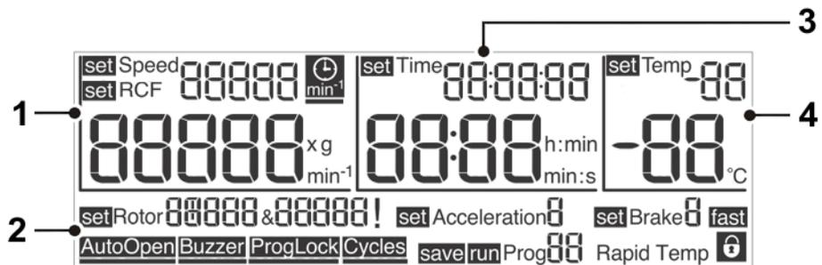
Fig. 15: Display of the Spincontrol L control system
