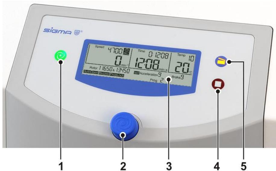
Fig. 14: User interface of the Spincontrol L control system
