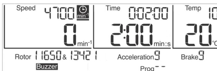
Fig. 18: The function "Runtime as of the set speed" is activated
