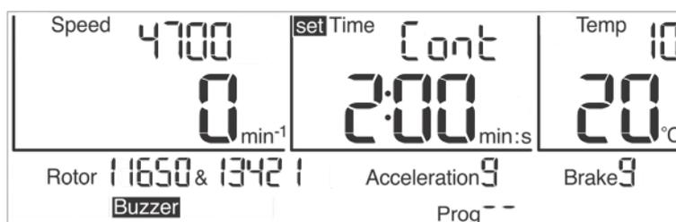
Fig. 19: Indication "Cont" during a continuous run
