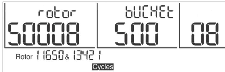
Fig. 29: Display when the maximum number of cycles is reached (flashing)
