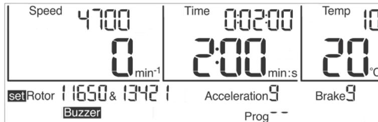
Fig. 23: Preselection of a rotor or a rotor/bucket combination
